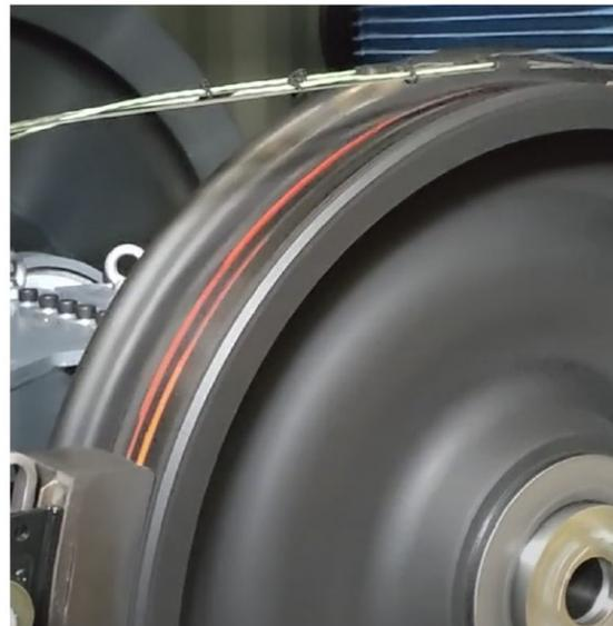
Image showing hot bands forming on the wheel treads, indicating that heat flux is not evenly distributed
