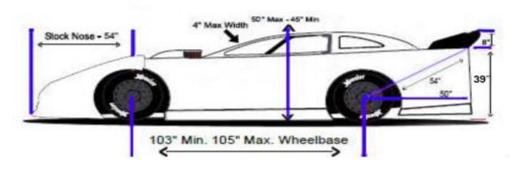
FRONT ROOF SUPPORTS 4" MAX. WITH 12" FLARE MAX. AT BOTTOM.
