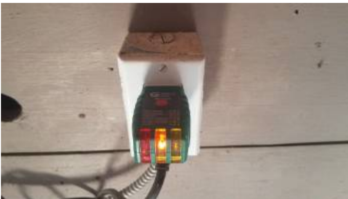
Receptacle Not Grounded In Garage
