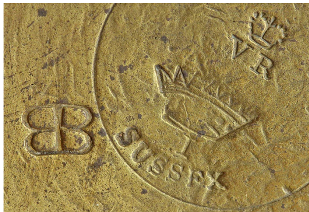
¶ Detail from a 1 lb brass weight, showing the non-uniform verification mark for the Borough of Bedford, together with the mark for the Lewes District of West Sussex.
