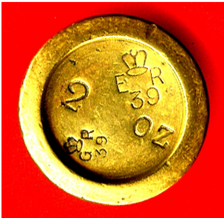
¶ A 2oz brass weight stamped with the uniform verification number (39) assigned to the Borough of Bedford. ER 39 indicates the reign of Edward VII (1902-1910) and GR 39 indicates his successor George V (1910-1936). Strictly speaking, the latter mark should have been stamped on the back of the weight, according to the regulations in force from 1907 onwards.
