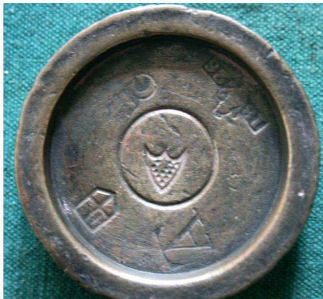
¶ This weight has several Cornish marks. The lowest mark, No.2 B DISTRICT, is probably from the period 1846-58 when Elias Liddell was the inspector for the Bodmin district. The weight has subsequently been adjusted with a copper plug and stamped with the mark for police district A (also Bodmin), used in the period 1858-1890. There is also the number 194, which was issued to the Borough of Bodmin in 1879. Finally there is a mark with the county number 9 issued in 1891.
