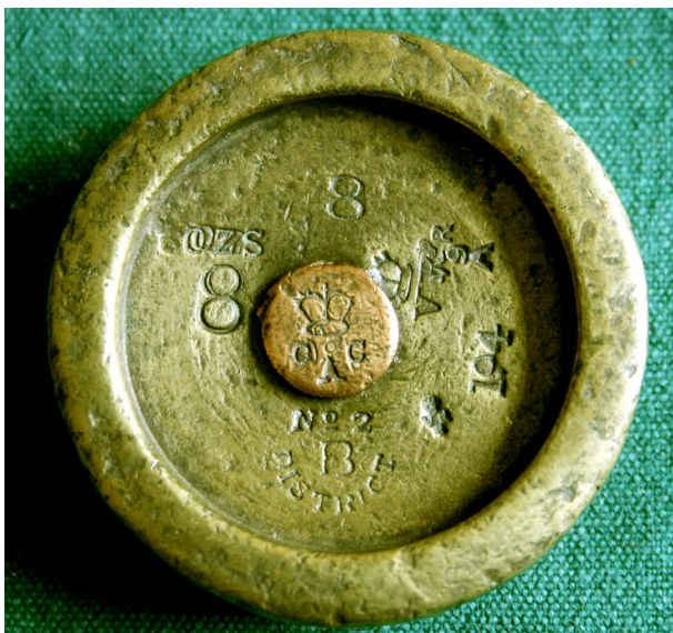
¶ This weight has several Cornish marks. The lowest mark, No.2 B DISTRICT, is probably from the period 1846-58 when Elias Liddell was the inspector for the Bodmin district. The weight has subsequently been adjusted with a copper plug and stamped with the mark for police district A (also Bodmin), used in the period 1858-1890. There is also the number 194, which was issued to the Borough of Bodmin in 1879. Finally there is a mark with the county number 9 issued in 1891.
