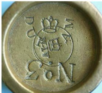
¶ Details from four weights, showing variants of the Durham County stamp, together with the divisional mark; the first weight also bears the quadrant mark of Sunderland, whilst the second carries a Northumberland County mark.
