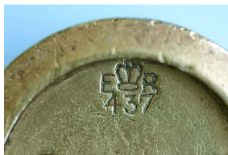
¶ Details from two 2oz brass weights, showing the VR437 and ER437 uniform verification marks for Stockton.
