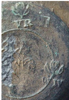
¶ Detail from a bronze 8oz weight, showing the Saffron Walden verification mark for both William IV (1830-37) and Victoria (1837-79); the detail from the 1 oz brass weight Shows the verification number for the Borough (1879-89).
