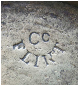
¶ A Flintshire verification mark stamped on a brass weight, probably in the period 1835-1858.
