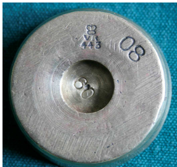
¶ Reverse of a brass weight stamped with the Flintshire number 443 in the years 1882-1901. The date marks refer to later re-verifications in 1908 and 1909.
