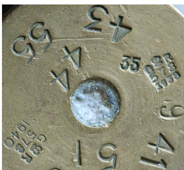
¶ Detail from a 2 oz brass weight, with the verification number GR578 for Merthyr Tydfil, together with stamps showing the years in which the weight was re-verified.
