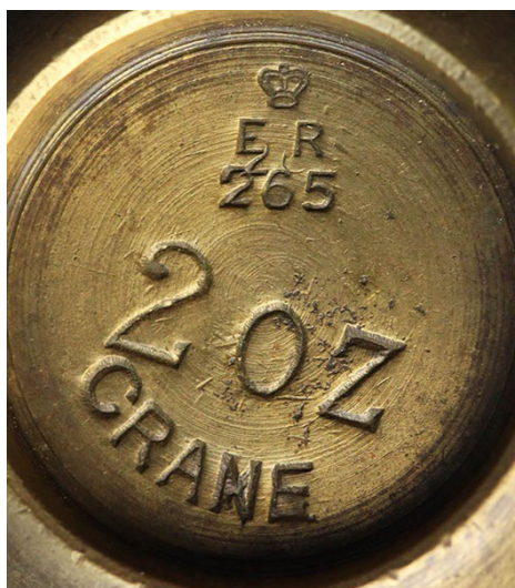
¶ Detail from a 2 oz brass weight, showing the uniform verification number for Southampton, stamped in the period 1901-10.
