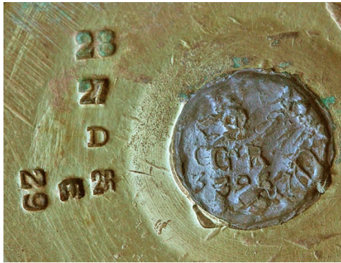
¶ Two details from the reverse of a 1lb brass weight by Walter Parry (see also Section C) showing the date stamps for 1926 - 29 and the GR395 mark of the Barnet Division.
