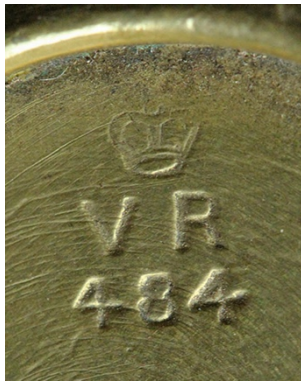
¶ Details from two 2 oz brass weights, showing the uniform verification numbers used in the East and West Divisions respectively, stamped during 1890-1901 and 1901-1910 respectively.
