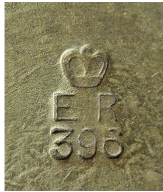
¶ Details from two 2 oz brass weights, showing the uniform verification numbers used in the East and West Divisions respectively, stamped during 1890-1901 and 1901-1910 respectively.
