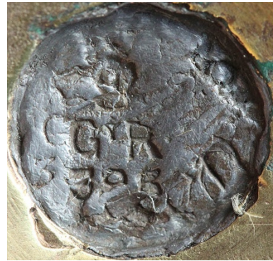
¶ Two details from the reverse of a 1lb brass weight by Walter Parry (see also Section C) showing the date stamps for 1926 - 29 and the GR395 mark of the Barnet Division.
