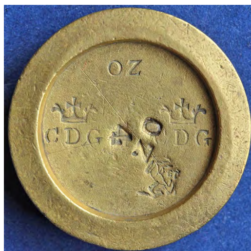
¶ A 4 oz brass weight, showing the verification mark for the Wingham District of Kent and the mark (?) of Charles Gould, the Inspector of Weights and Measures for Canterbury 1863-69.
