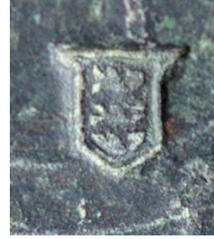
¶ A 2 oz bronze weight, dating from the reign of Charles II, bearing both the non-uniform mark and the verification number for Sandwich, together with a detail of the non-uniform mark.
