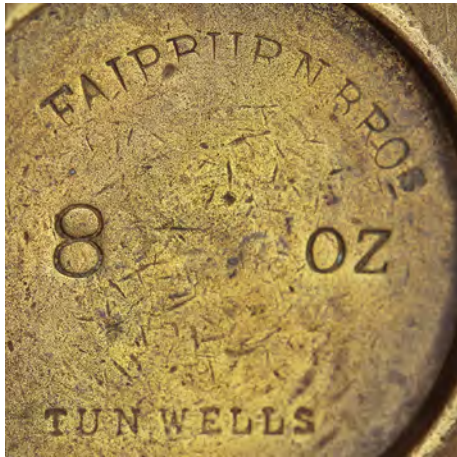
¶ Detail from an 8 oz brass weight; the verification mark in the lead plug on the reverse shows that it was stamped in Tunbridge Wells in the reign of Edward VII (1901-10).
