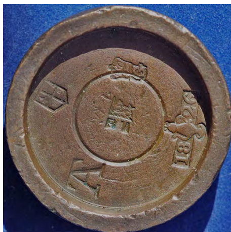
¶ A 2oz bronze weight bearing the London Founders marks (1826-30) and the non-uniform verification mark of Margate (1869-1879).
