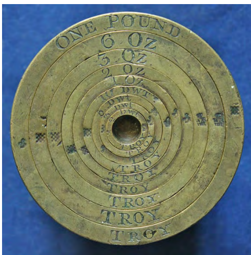
¶ The set of Troy-weight standards for Queenborough from 1835, with the modern spelling of the name being engraved on the reverse.
