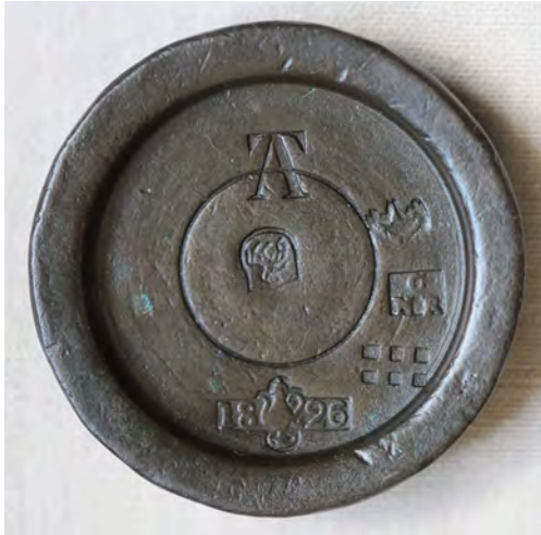
¶ An 8 oz bronze weight, originally stamped in London, showing the three stamps of New Romney, together with the mark of District 9, Ashford (1834-66).
