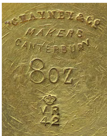
¶ Detail from an 8oz brass weight, by Chayney & Co, Canterbury; the weight has been verified in the City of Canterbury (VR42) in the period 1894-1901.
