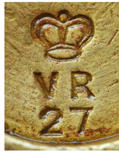
¶ Details from two 1 oz brass weights showing the non-uniform verification mark (1835-1879) and the VR27 mark (1880-1901) of the Borough of Maidstone.
