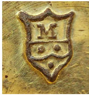
¶ Details from two 1 oz brass weights showing the non-uniform verification mark (1835-1879) and the VR27 mark (1880-1901) of the Borough of Maidstone.
