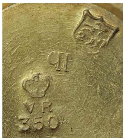
¶ Details from a ½ lb bronze weight, a 2oz and a ¼ lb brass weight, showing the verification numbers in use 1880-1906. The last one also carries the old mark for District 2.
