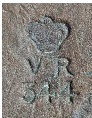
¶ Details from a ½ lb bronze weight, a 2oz and a ¼ lb brass weight, showing the verification numbers in use 1880-1906. The last one also carries the old mark for District 2.
