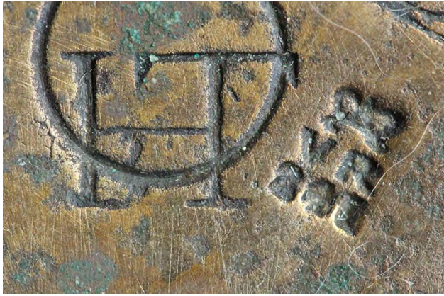
¶ Detail from a ½ lb bronze weight, stamped in the reign of William IV (1830-37), showing the non-uniform verification mark, with the initials of the inspector Benjamin Hatch and the T of Tenterden, together with the VR241 mark of the borough of Tenterden (1879-89).
