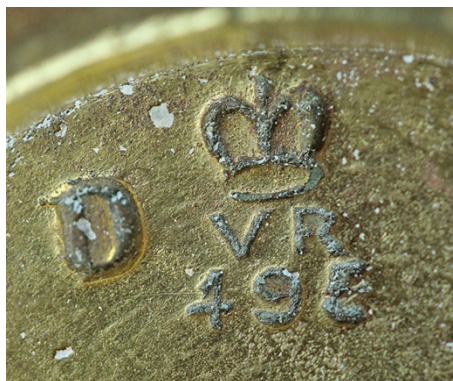
¶ Detail from the 4oz brass weight, shown above with the 1870 and 1873 marks, but this time stamped after the adoption of the uniform verification number (1889) and with a letter code replacing the date of the examples above.
