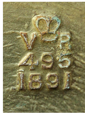
¶ Details from two 4 oz brass weights, showing the uniform verification number, but maintaining the tradition of showing the year and an altered format.
