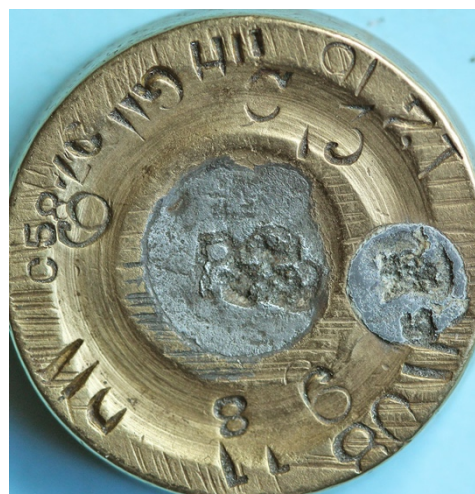
¶ A 1 oz brass weight stamped in Blackpool. The first detail shows the VR533 (1892-1901) and the ER533 (1901-1910) marks, whilst the second one illustrates the various systems of dating used.
