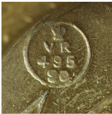
¶ Details from two 4 oz brass weights, showing the uniform verification number, but maintaining the tradition of showing the year and an altered format.
