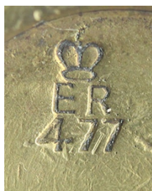
¶ Detail from a 2 oz brass weight, stamped with the uniform verification number of Burnley
