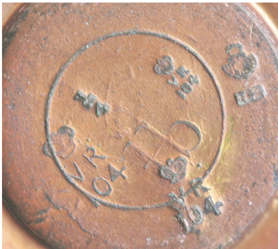
☪ Detail from a ¼ lb brass weight, showing the VR104 verification mark of the Bootle division, stamped in the period 1879-1901; the weight also carries the mark of the City of Liverpool, with the date stamp H2.
