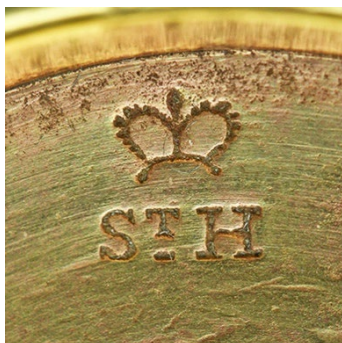
¶ Detail from an 8 oz brass weight, with the non-uniform mark for the borough of St Helens, together with the stamp from a lead plug, showing the verification number and a date code.
