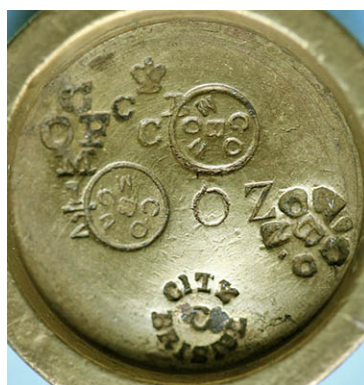
¶ A ½ oz brass weight, showing the original County mark, the mark for the A district of the County (Pontypool), and one for the City of Bristol.
