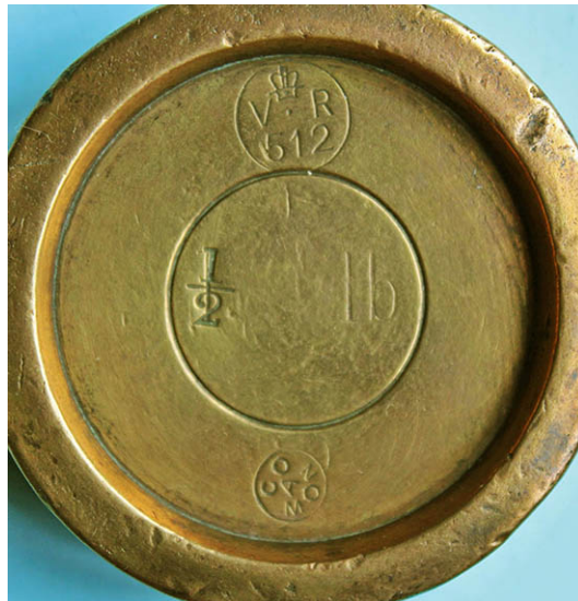
¶ A ½ lb brass weight, with the marks for the Abergavenny district of the County and the later uniform verification mark 512.
