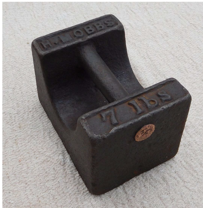
¶ A 7 lb iron bar weight made at Henry Mobbs' Lion Foundry in Northampton, c.1870-80. The copper plug has the verification mark of Holland in Lincolnshire.
