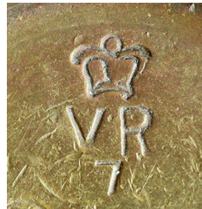
¶ Above: detail from a 2oz brass weight showing the verification number 7 for Nottingham, 1879-1901.
