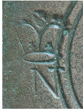
¶ The early form of the verification mark, on a bronze 4oz weight. The only marks on the weight are two identical stampings, as above.
