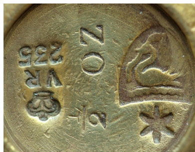
¶ Detail from a ½ oz brass weight, showing the cormorant mark, used in Newark in the period 1834-78, together with the uniform verification mark 235
