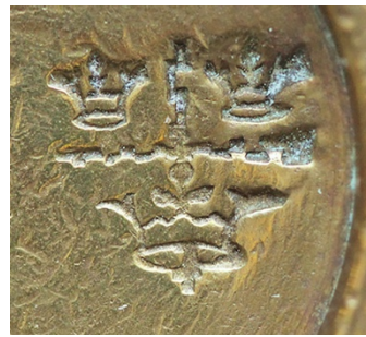
¶ Details from two weights stamped in Nottingham in the period 1834-78. The first is from a bronze 2oz weight, the second from a brass 1oz one.
