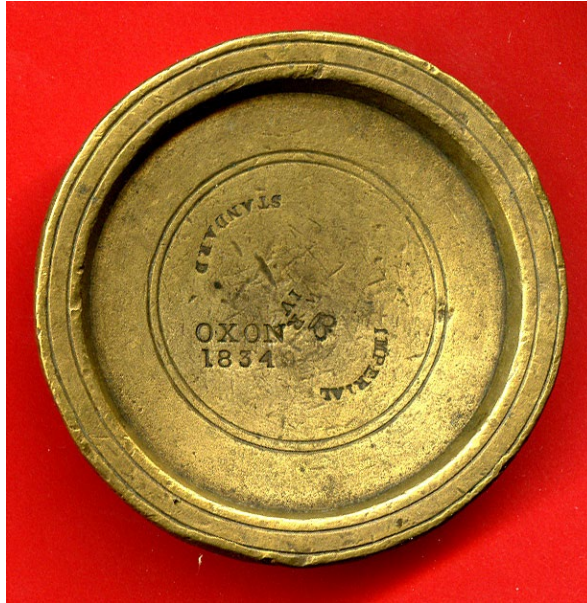
¶ A 1lb brass weight stamped in Oxfordshire by one of the inspectors appointed in 1834. The other marks are stamped by the maker (probably a Birmingham firm) and indicate that the weight was made in the reign of William IV (1830-37) and conforms to the Imperial Standard.
