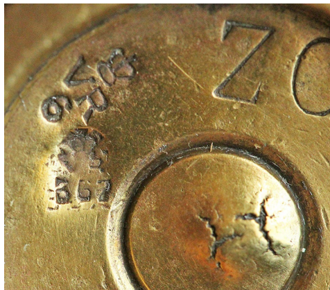
¶ Detail from a 1 oz brass weight, showing the uniform verification number VR367 (1880-1901), together with the VR6 of Birmingham. The reverse shows many date codes of the form G8.
