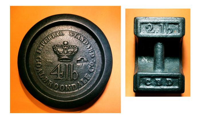
¶ Two weights from the Coalbrookdale Company. The one on the left has been verified in the 'Borough' of Wenlock, in which the foundry was situated.
