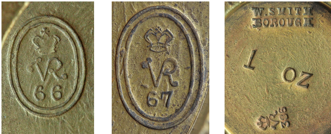
¶ Details from three brass weights, 2 oz, 1 lb and 1 oz respectively, showing the uniform verification numbers that were transferred to the LCC in 1889.
