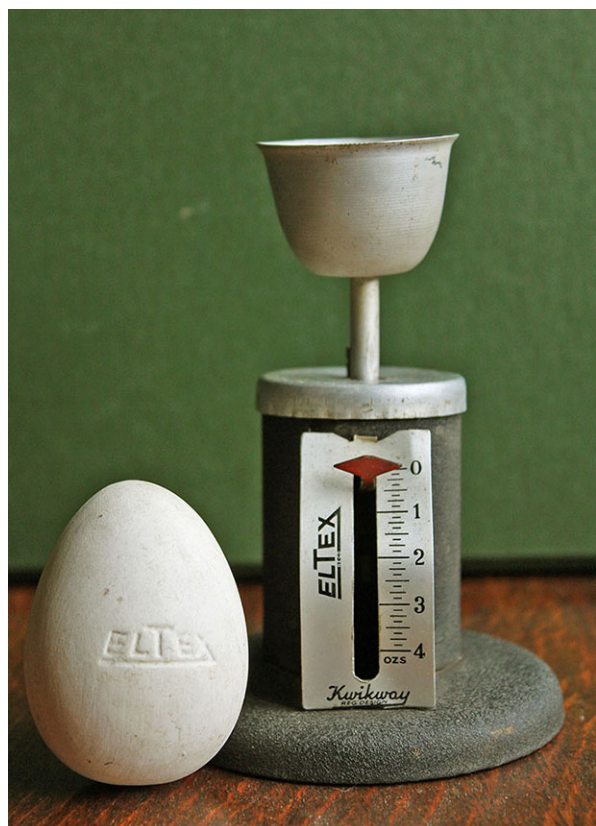
¶ The Eltex/Kwikway egg grader (with artificial egg for demonstration purposes) and an advertisement for the firm, mentioning Pig Weighing Machines.
