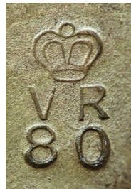
¶ Detail from a 2oz brass weight, showing the uniform verification number for Scarborough.
