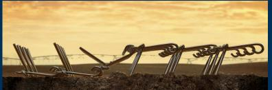
Dual Action: Front section aggressive action, rear section levels.
