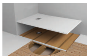
or included at joist level (decks should be fully supported by creating a false floor between joists)
