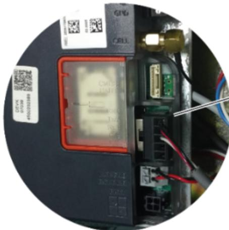
**Disconnect the RS232 connector from the Cloud Link 4G Modem.**
