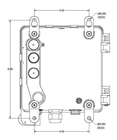
Figure 5-1: Wall Mounting Tabs and Dimensions
