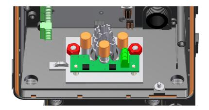
Figure 9-2: Pulse Output Board
