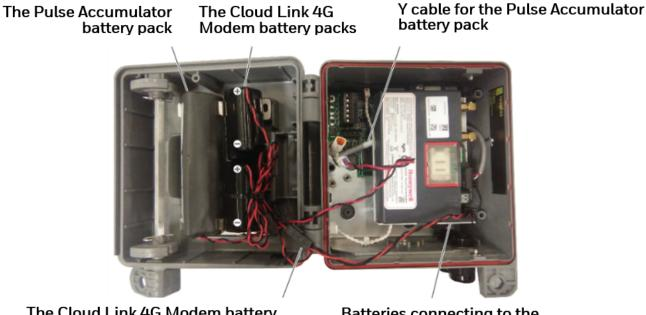
The Cloud Link 4G Modem battery packs connected in parallel Batteries connecting to the Cloud Link 4G Modem
