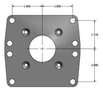
Figure 5-4: Universal Mounting Bracket (UMB) Hole Pattern
