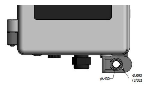
Figure 7-2: Enclosure Sealing Options
