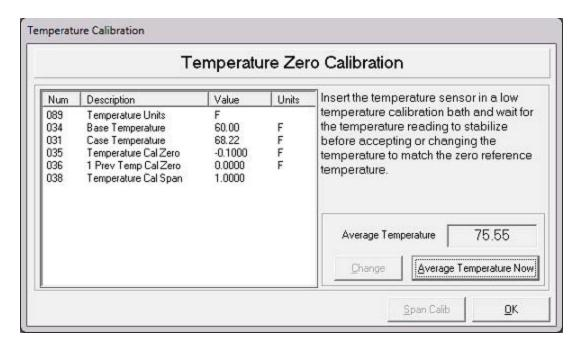
2. Insert the temperature probe of EC 350, along with an accurately calibrated thermometer calibrated thermometer into a low temperature bath or dry well, which provides the temperature zero reference.
