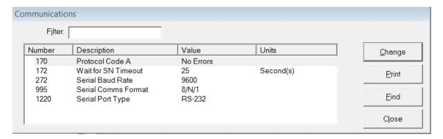
Items 170 and 172 are primarily associated with the behavior of MI Protocol. These should normally left as default (shown here). The remainder will vary depending on the external devices. See also Modbus section below for settings relevant to the Modbus protocol.
