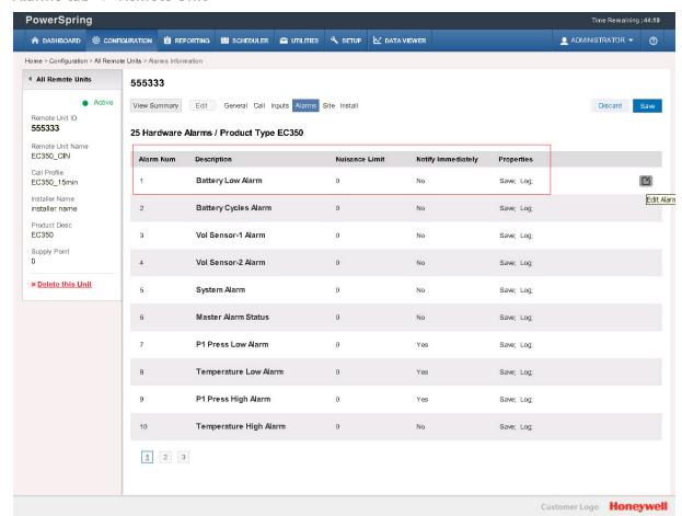
Navigate to ALARMS tab as and configure the ALARMS for EC 350 device, user can configure the alarms thathe wants to display in PowerSpring Alarm/System Monitor application. As shown below user has to EDIT the existing alarm.
