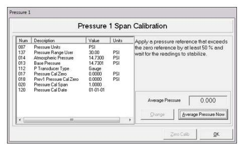
8. Apply a high pressure such that the pressure applied is at least 50% more than the zero reference pressure.
