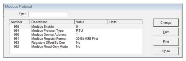
If the external device communicates via Modbus protocol, item 985 must be set to 1. Item 994 will need to be set to the proper Modbus variation, either RTU or ASCII. The correct setting for all of these items will be determined by the external device used.
