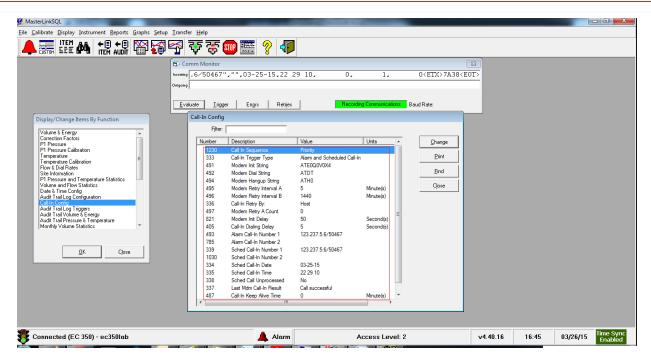
9. Type the information as shown, items: 1230, 333 (you may choose some other item numbers as well, 491, 492, 494,495, 496, upto last). Critical items are, 339 & 493, where the Host machine's IP Address for MERCURYSERVER and TCP Port (50467) should be correctly specified. The remaining fields can be defined by the user.
