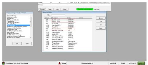
PowerSpring can use Site ID 1 or Site ID 2, that is setup in **System Configuration -> Data Collection settings**. The default is Site ID 2.
