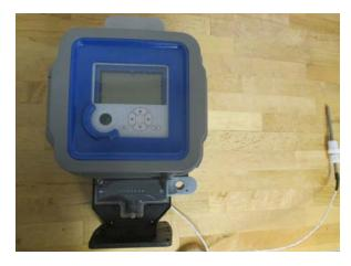
• Installing EC 350 on a rotary mount. The following image illustrates EC 350 configured for a rotary mount. (Adapter plate, which varies by meter model, not shown.)
