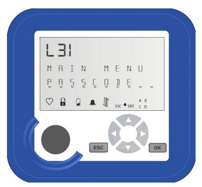
3. To access the passkey screen, in level 3 mode press **OK**. The following appears on the display. 0000000
