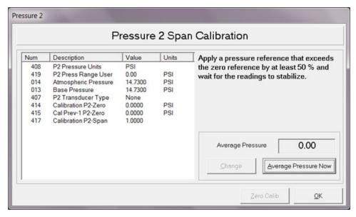
9. Apply a high pressure such that the pressure applied is at least 50% more than the zero reference pressure.
