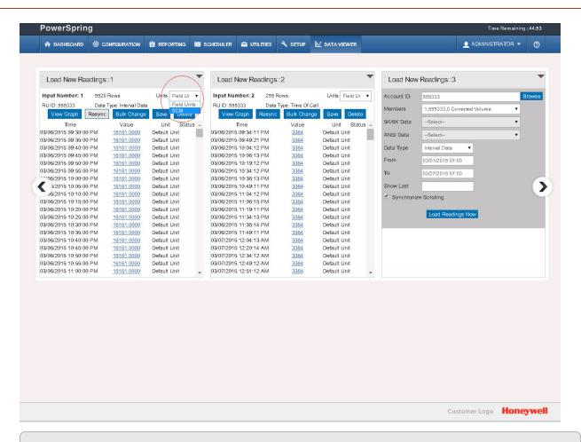
**Note:** The Operator and Factors given for the REPORT or FIELD UNITS should be used correctly in DATA VIEWER. In the below screenshot user can see the SCM report unit contains the Operator1=\* and Factor1=10. It means the multiplication by 10 should be done in data viewer, if user displays the data in data-viewer application for report unit selected as SCM.
