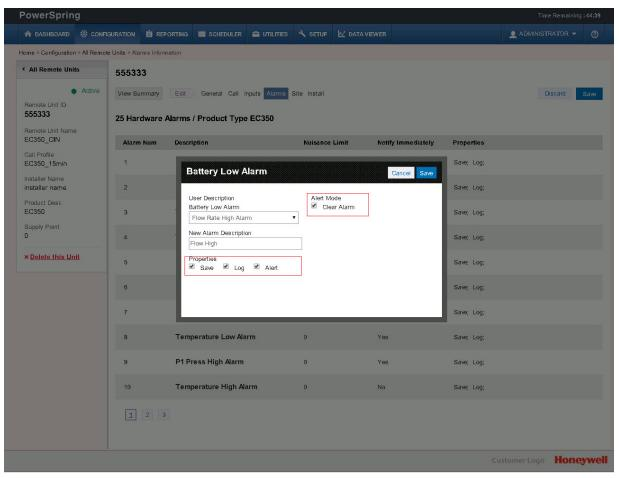
Use this tab to edit the Remote Unit Hardware Alarms' information. However, there are certain hardware alarms that are "non-maskable;" that is, the hardware alarms are always active and you are only permitted to customize the name (user description). When you select one of these hardware alarm types, (from the Hardware alarm list), the Immediate alarm notification check box and Nuisance limit box, (under Alarm Specification), appear dimmed and are unavailable for modification.
