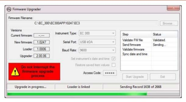
8. After the upgrade is complete, **Upgrade was successful** (in green) appears at the lower left corner of the main **Firmware Upgrader** dialog box.
