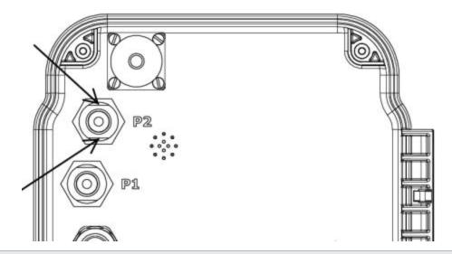
Warning: To avoid explosion, it is extremely important to ensure the pressure transducer is capable of handling the pressure in the gas line. Check item entry 137 (user units) or item entry 25(PSI) on the EC 350 for maximum pressure transducer information before applying live gas pressure to the EC 350.
