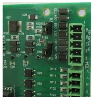
For RS-232, only 3-wire communications is supported: pin 1 TXD (Transmit Data), pin 2 RXD (Receive Data), and pin 5 GND (Ground). (The TB4 RTS/CTS connections are not used.) TXD and RXD are labelled as a DTE device (EC 350 transmits on TXD).
