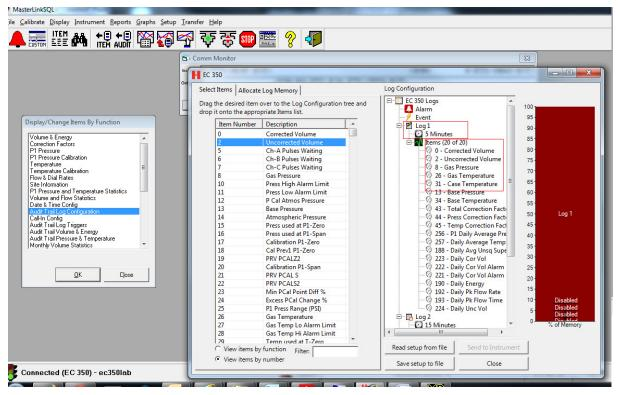
3. Call-In Configuration: Inside the **Display/Change Items By Function** sub-window, double click on **Call-In Config** option. Enter the information as shown in the region marked in red. i.e. items 1230, 333, 491, 492, 494,495, 496, upto last – depending on how the user wants the Callin to happen.
