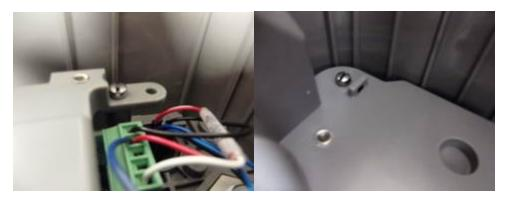
3. Re-install Human Factor cover tightening the screws to 9 + / - 1 in-lbs of torque at these locations. Ensure power cable is routed in the orientation shown for battery connection.
