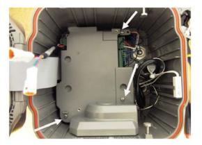
2. Using sealing wire and lead seal, seal cover at these locations. Run wire through the screw head, and then through the MC cover sealing features.
