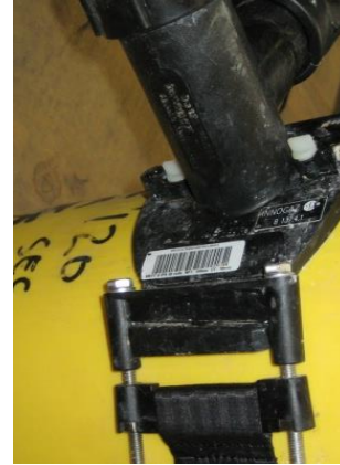
Incorrect clamping of belt strap
