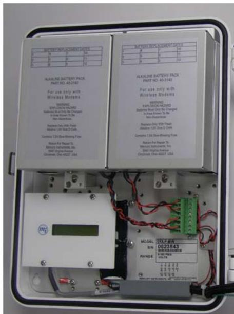
**Figure 32: Quad Battery Pack**
