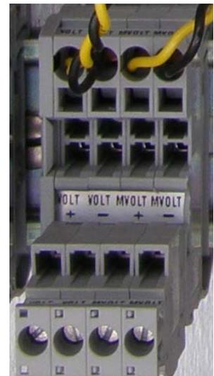
To operate the CPRI board, determine the full scale rectifier voltage and current shunt millivolt ranges and set the jumpers on the CPRI board accordingly. Note that the measuring range in the ERX is 80% of the jumper selections.
