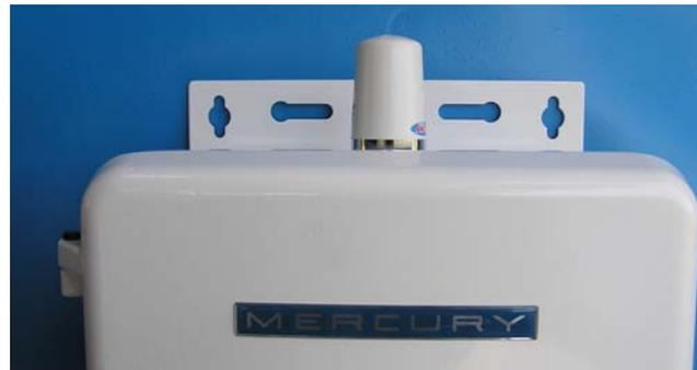
Figure 8: Case-mounted Antenna
