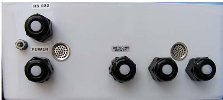
There is a cable grip on the bottom of the assembly box to run the TEC2 cable through. It is labeled "power". There is an additional cable grip for wiring power out to an external device labeled "outgoing power". Make the appropriate connections at the remote charger, as described in the next section, and then wire into the MI Wireless assembly as below.
