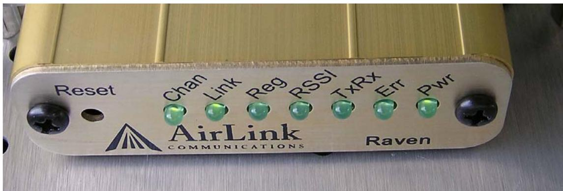
Figure 60: CDMA Modem LEDs
