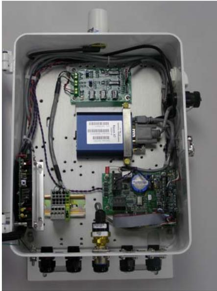
two pressure inputs on your ERX board as electrical monitoring inputs and is available in Quad-Alkaline, Solar, and AC-powered configurations. There is one voltage input that can be used for pipe to soil or rectifier voltage. The millivolt input can be used for rectifier current. A rectifier control option is also available in AC powered assemblies.
