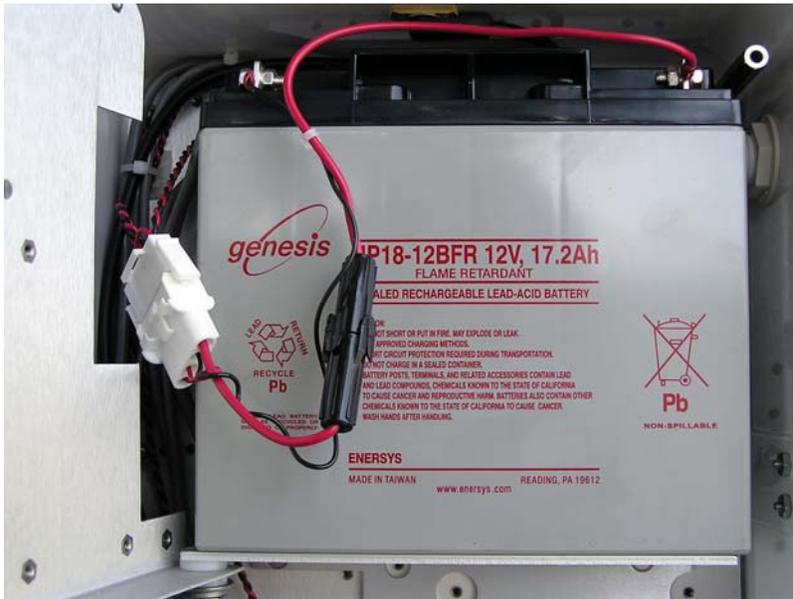
Figure 14 Battery, Connector, and Fuse
