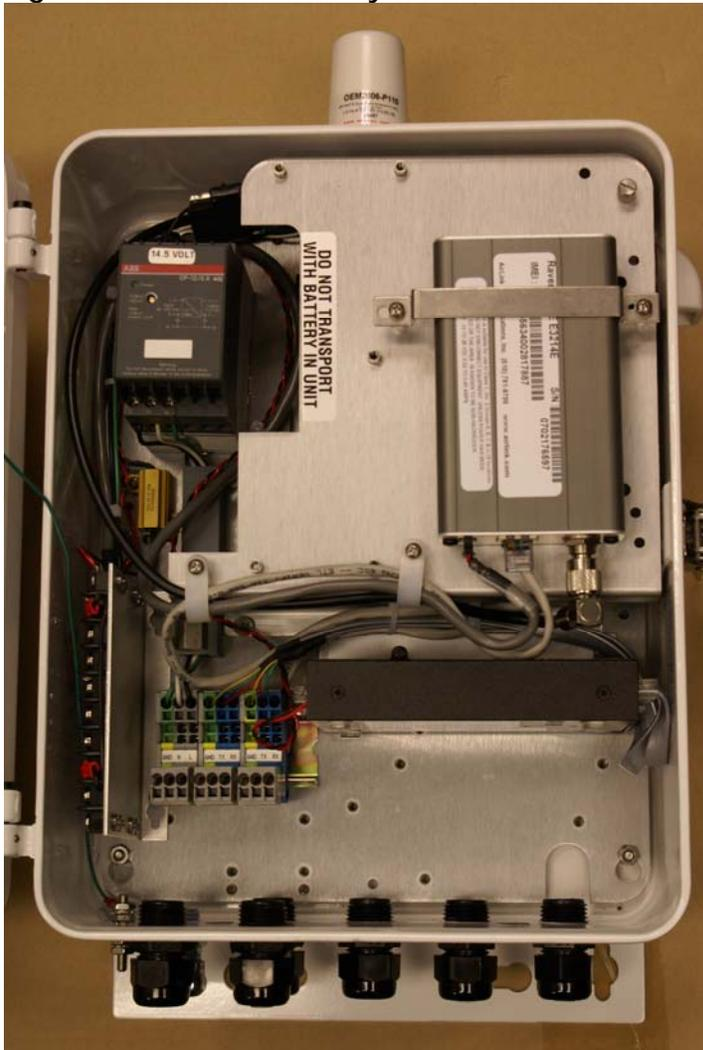
One serial terminal block is available in the lower left corner of the assembly for each serial output. Cable grips for each serial cable are available in the bottom of the assembly.
