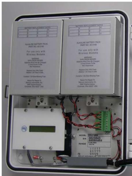
**Figure 32: Quad Battery Pack**
