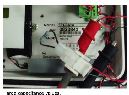
To check the function of the capacitor in the field, disconnect the capacitor from the rest of the system and measure the capacitance with a digital multi-meter. While capacitance will degrade over time, the capacitance should be 2.5F within 20%. Make certain that your meter has the ability to measure
