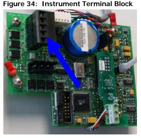
data output connectors on the MIW assembly. This is shown by the blue arrow in the figure. This terminal block + and – connectors should be wired to the A+ and A- terminals on the Mercury ERX or Mini-Max instrument TB1. On the Mini-AT, the terminal block - and + connectors should be wired to J20 Aux Modem pins 2 and 4 respectively.
