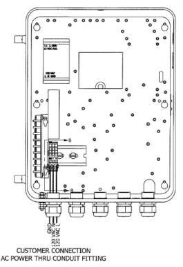
Make the appropriate connections at the AC supply, and then wire into the MI Wireless assembly as below.
