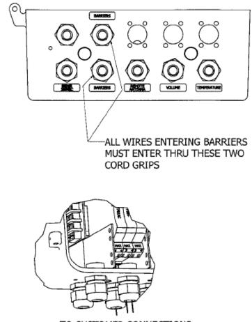
TO CUSTOMER CONNECTIONS Figure 35: Wiring into enclosure made by someone other than the person(s) who carried out the installation work. For questions, refer to the appropriate authorities in your area.
