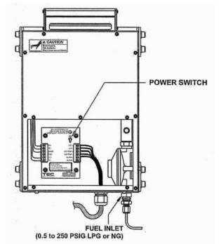
The TEC-2 comes with a Battery Interface Module to interface the TEC to the external battery that it will keep charged. The TEC will not start with a "dead" battery. In order for the TEC to start, the remote battery to be used must measure greater than 11 volts. The Battery Interface Module contains a temperature sensor and an over-current protector and should be located near the battery being charged. The charging set point of the TEC2 is controlled by the diode temperature sensor.
