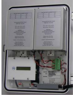
Figure 32: Quad Battery Pack
