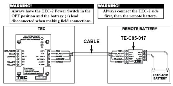
Figure 23: TEC-2 Cabling
