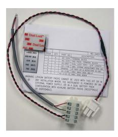
from the tape on the terminal strip and attach to inside wall. Press firmly. Carefully remove terminal strip by separating dual lock tape. Connect field wiring to terminal block Com, RxD, and TxD. Run wires carefully over to MI Wireless assembly and wire to Com, RX, and TX, respectively. Make certain that the wires to not interfere with closing of the door. For details, consult the included instructions 40-3401-A.
