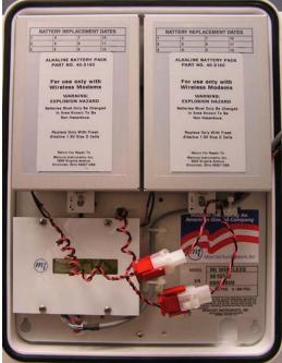
Figure 31: Dual Alkaline Assembly
