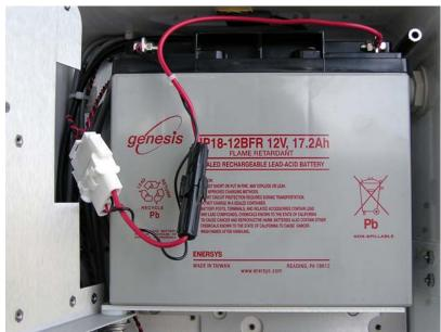
Figure 14 Battery, Connector, and Fuse
