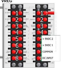
"+", and "-". The positive leg of the remote equipment should be connected to "+" and the negative leg should be connected to "-". See wiring diagram on customer connection drawings or in picture below.
