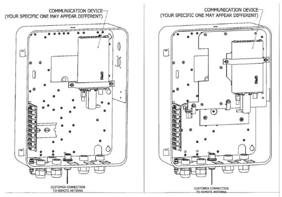
Figure 10: Remote Antenna Installation Diagram
