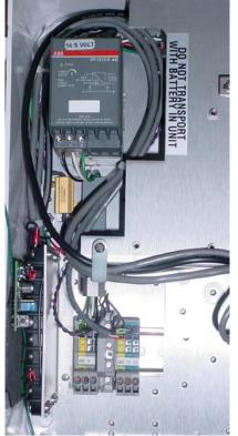
The AC Hybrid power source includes a 12VDC adjustable power supply, 7AH rechargeable sealed lead acid backup battery, and SunSaver Solar Controller. The power supply will look similar but may not be identical than the one in Figure 24: AC Power. The 12VDC power supply is adjusted to 14.5VDC to provide optimum power to the SunSaver Solar controller to charge the battery. The SunSaver Solar Controller and battery are located behind the pivot panel.
