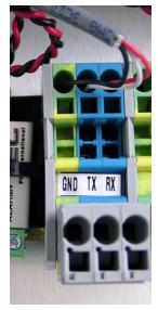
If your MI Wireless Assembly does not include an internal instrument board, the MI Wireless modem connection is available on the terminal internal connections. The Messenger Modem GND, TX, and RX should be wired straight through to the GND, TX, and RX of the part number 40-1074 or 40-2717 terminal blocks.
