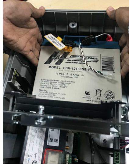
3. Connect the battery pack cable (\*) to battery charge controller cable.
