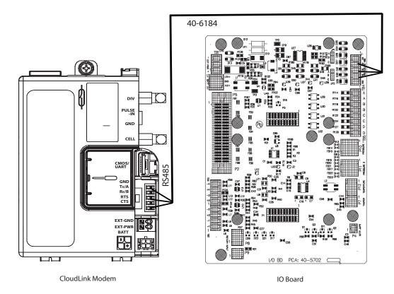
Figure 5-3: Electrical Wiring between IO Board and CloudLink Modem
