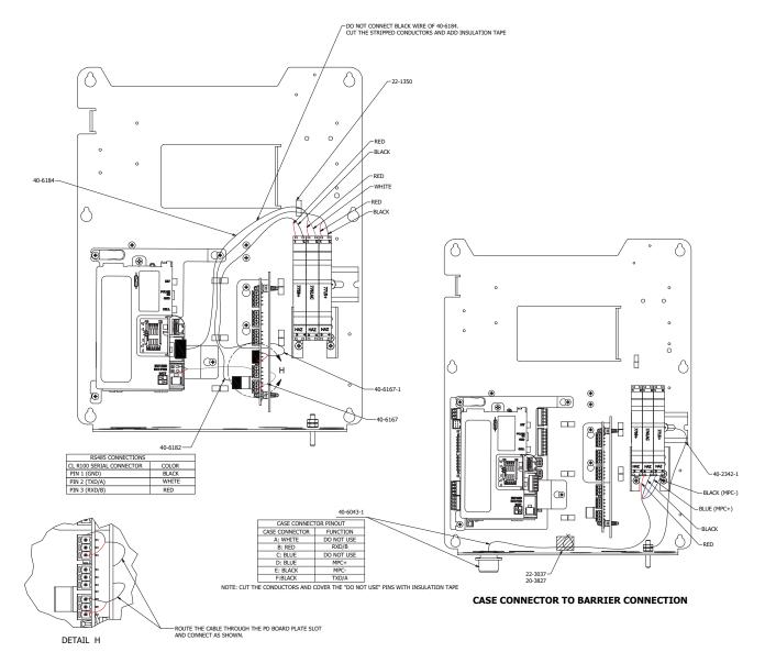
Figure 7-5: Internal Wiring - CloudLink R100 Connections
