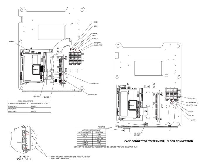
Figure 7-9: Internal Wiring - CloudLink R110 Connections
