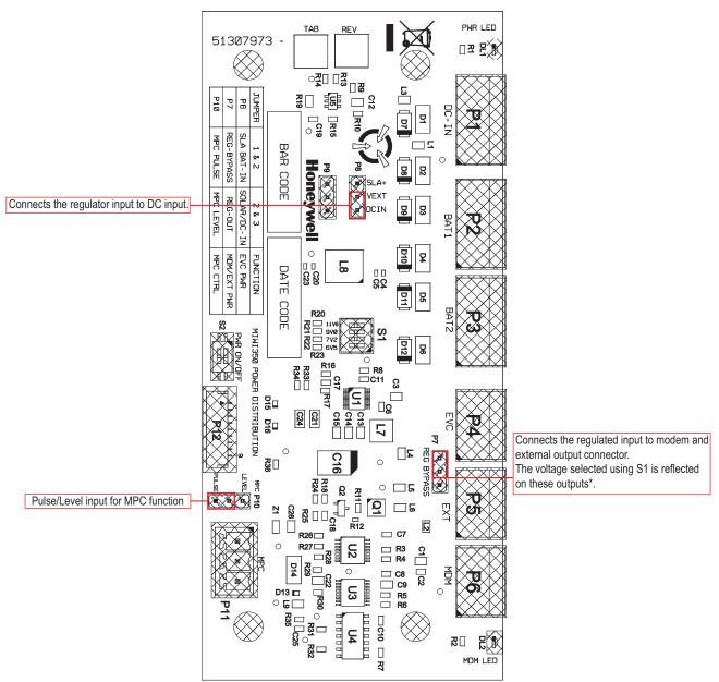
\* **IMPORTANT NOTE**: Never exceed 9V for Alkaline battery input. The supercap connected cannot work beyond 9V.
