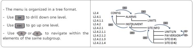
Refer to the Honeywell EC350 User's Manual for more information on using the HMI User Interface.
