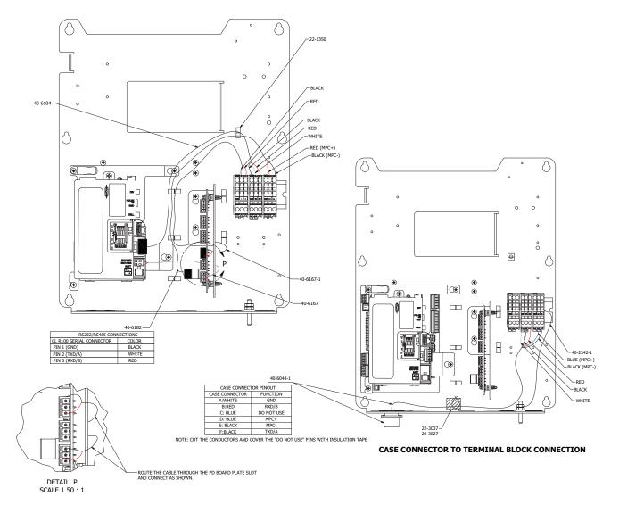
Figure 7-8: Internal Wiring - CloudLink R100 Connections
