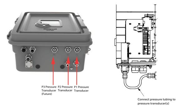
Follow the below steps to connect pressure tubing to pressure transducer(s):
