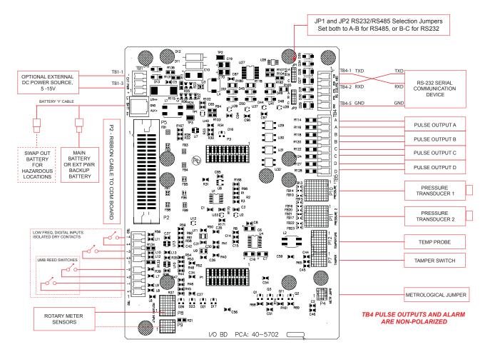
Figure 4-1: Input/Output Board or EVC Board
