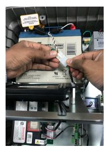
2. Carefully insert the battery in the mount bracket.
