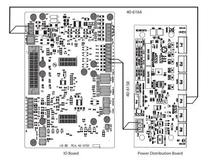
Figure 5-1: Electrical Wiring between Power Distribution Board and IO Board
