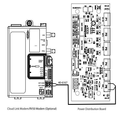
Figure 5-2: Electrical Wiring between Power Distribution Board and Modem
