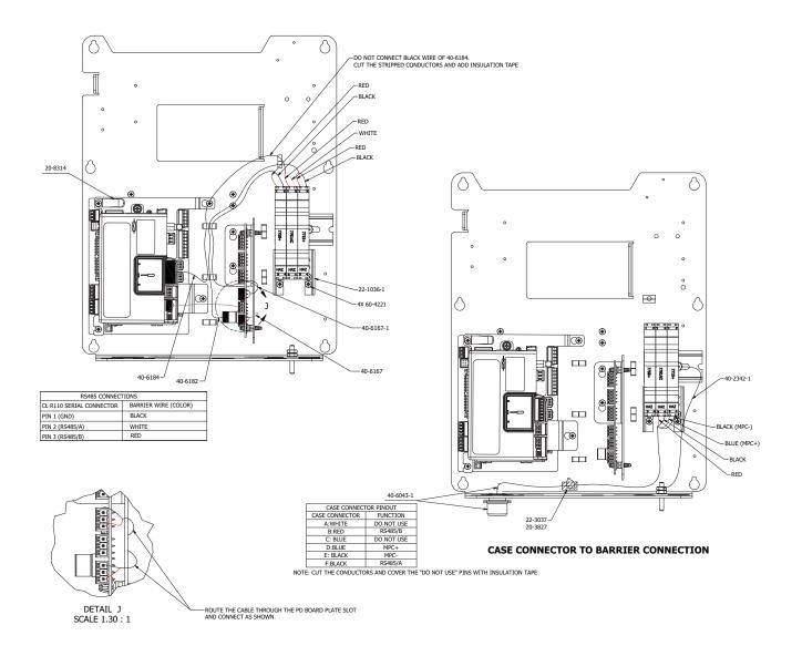
Figure 7-6: Internal Wiring - CloudLink R110 Connections
