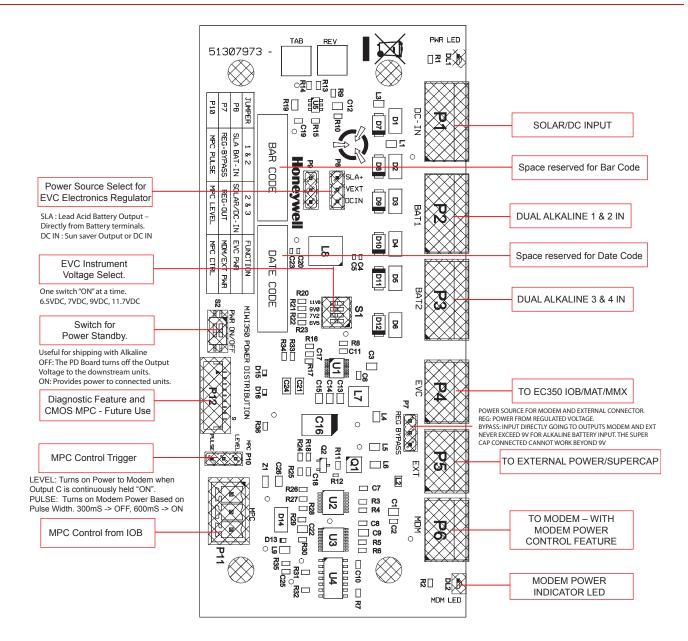
Figure 4-2: Power Distribution Board
