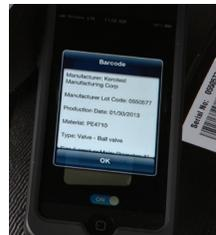
All POLYBALL valves now feature the new industry standard tracking and traceability code per ASTM F2897 that allows instant access to individual valve specifications. With decoding software, simply scan the bar code to see the production date, size, material and valve type, lot code and more.
