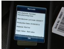
All POLYBALL valves now feature the new industry-standard tracking and traceability code per ASTM F2897 that allows instant access to individual valve specifications. With decoding software, simply scan the bar code to see the production date, size, material and valve type, lot code and more.
