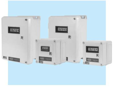
\*NEMA 4 enclosures are intended for indoor and outdoor use. They provide protection against windblown dust, rain, splashing and hose directed water. The fiberglass reinforced polyester construction allows the product line to be nonconductive, lightweight and impact resistant.
