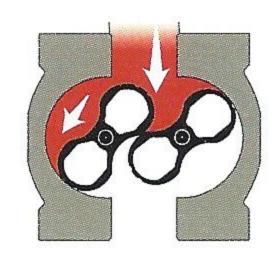
As the left impeller rotates toward the vertical position, gas enters the cavity created between the impeller and the housing.
