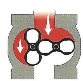
When the left impeller reaches the vertical position, a finite volume of gas is captured in the left cavity.
