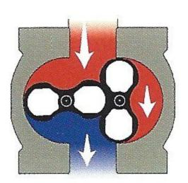
After further rotation, the right impeller becomes vertical and a finite volume of gas is captured in the right cavity.
