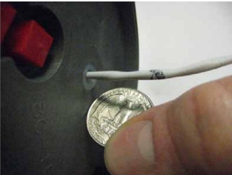
Temperature probe marked 1" from mounting plate
