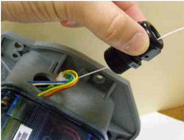
4. If field pulse cable is smaller than 0.2" diameter, install rubber tube supplied with unit onto cable such that the strain relief will clamp onto the tube once re-installed.
