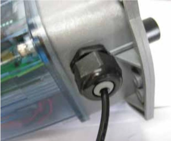
ⓘ The strain relief fitting contains a small hole drilled into the hex surface of the nut. This hole will accommodate a sealing wire for tamper sealing, if warranted.
