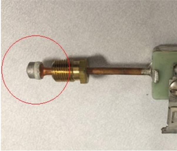
Above: this point of contact needs to be firmly seated. Same goes for the contact on the thermocouple.
