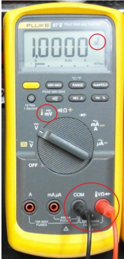
The AC/DC indicator is circled on the display screen. The yellow button switches between AC & DC on a Fluke meter like this. We need to take these readings in DC, so make sure that's displayed on screen.
