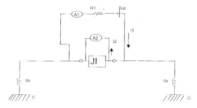
The following method of checking insulating joints consists in measuring the current I2 by means of an amperometer A2 in dry conditions.
