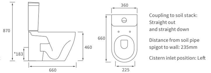
**RIMLESS CLOSE COUPLED PAN AND CISTERN FULLY SHROUDED
