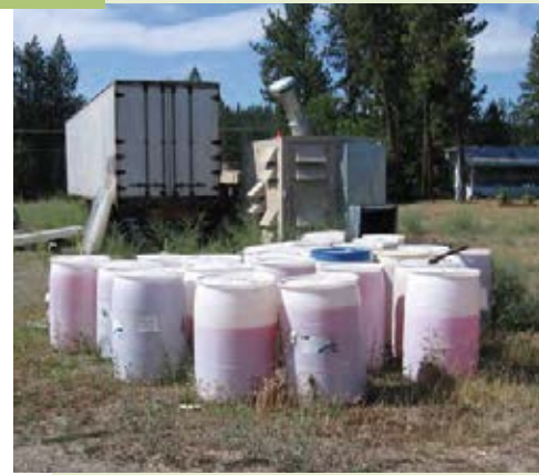
Chemical containers outside, without proper containment
