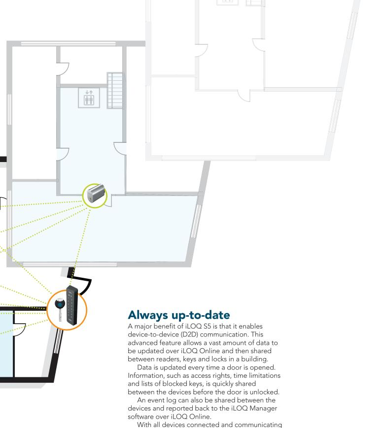
with each other, iLOQ S5 ensures that access rights are continually kept up to date. It reduces administration by removing the need to manually import or export data to locks or keys on-site using a programming device, not to mention the eliminates the hassle involved with mechanical locking systems when, for example, a key gets lost. It also minimizes the expenditure associated with system wiring and drives down lifecycle costs.
