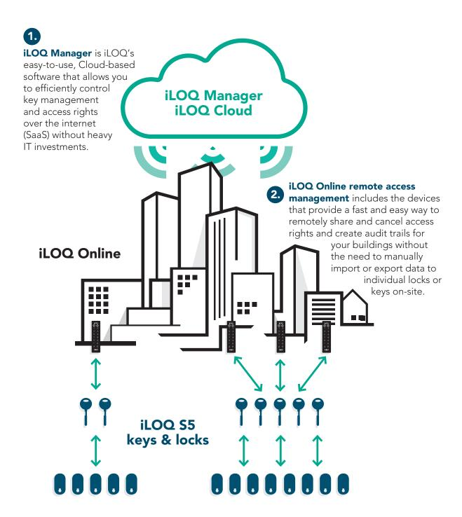
**3. iLOQ S5 keys and locks** are programmable. They can be reused and securely reprogrammed according to any changes in access rights, making the system easy to expand. Device-to-device communication allows a vast amount of data to be updated over iLOQ Online and then shared between the readers, keys and locks in a building.
