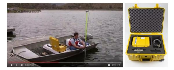
**Eliminate the need for a Separate GNSS Receiver.** There is no requirement to separately manage GNSS receiver operation and data communication with the acquisition PC. GNSS data are seamlessly merged with echo sounder data in the CEESCOPE<sup>™</sup> with little or no operator involvement needed to configure the GNSS. This reliable, easy to use, and accurate solution minimizes potential downtime and means you are set up and ready to survey as soon as the "on" button is pressed.
