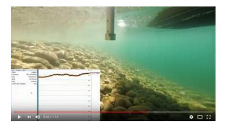
**Use AUTO or MANUAL Operation Mode.** For maximum control over the survey, the CEECOPE<sup>™</sup> may be used in AUTO or MANUAL mode. In AUTO mode, all echo sounder parameters are adjusted automatically to achieve the best results for depth and water column data. MANUAL mode allows the user to fine tune the CEESCOPE<sup>™</sup> to provide the best results for any survey feature, such as avoiding vegetation effects or tracking a sub bottom surface in dual frequency operation.
