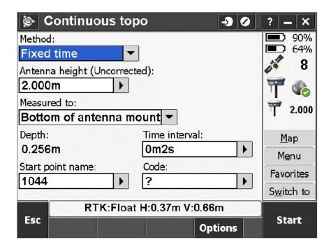
The antenna height is the distance from the GNSS antenna to the bottom of the transducer. The static draft (distance from the water surface to the transducer face) should be measured and noted.
