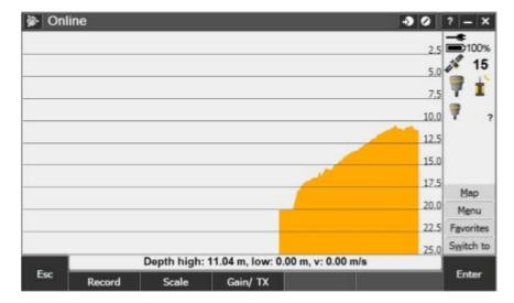
Pressing "record" starts a continuous topo measurement.
