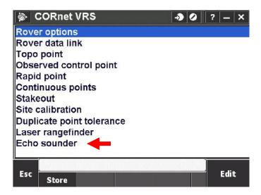
The echo sounder type is selected, in this case the echo sounder name is defined by the output data format. For the CEE LINE it is convenient to use NMEA SDDBT (NMEA Depth Below Transducer) generic device.
