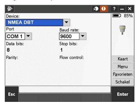
After the echo sounder is configured, the data collection method may be set up. Performing hydrographic surveys calls for a Continuous Topo measurement method usually based on a defined time interval (use the shortest possible). As the CEE LINE outputs data at 10Hz, there will be a depth measurement available every 0.1s.
