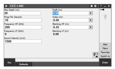
After the configuration is complete, the online screen may be used to view the sounding detail.
