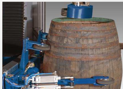
Flexible automatic clamping device for cask.
