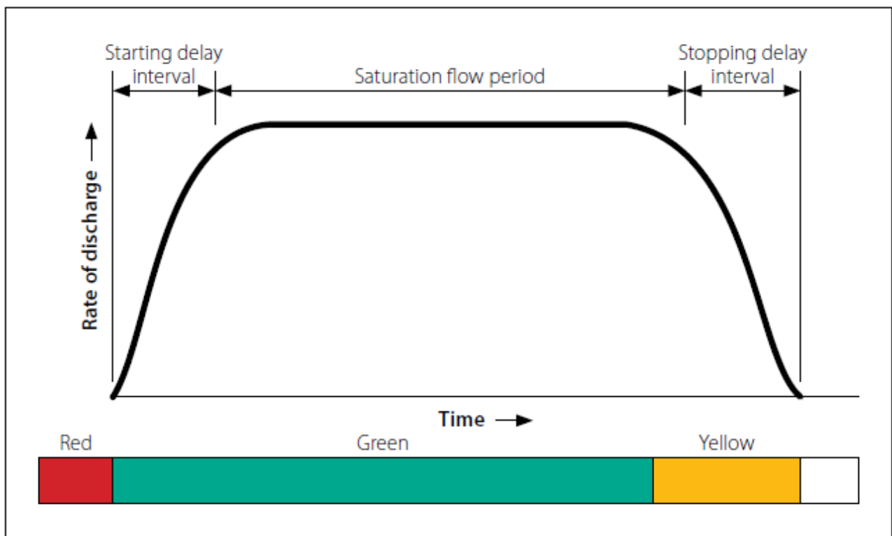
Figure 11: Discharge flow pattern across the stop line of a traffic signal illustrating start and stop delays
