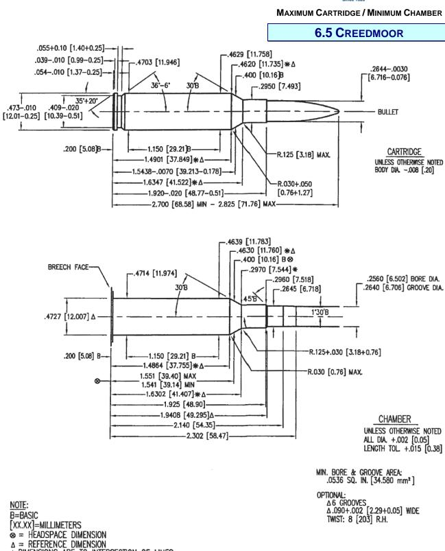
\* DIMENSIONS ARE TO INTERSECTION OF LINES ALL CALCULATIONS APPLY AT MAXIMUM MATERIAL CONDITION (MMC)
