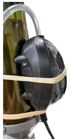
Air Pump on Dillon Powder Measure (Photo courtesy of Peter Griffin.)
