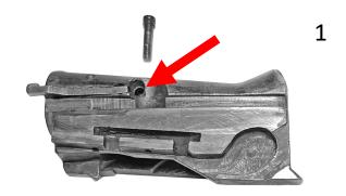
2. Remove firing pin retractor and spring. Remove original firing pin. These pieces will not be used.
