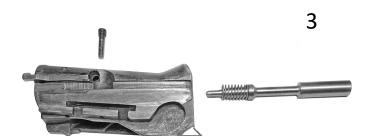
3. Install new firing pin and spring into bolt and make sure firing pin floats freely and does not stick. Some bolts have a burr around the firing pin hole that needs to be removed with a small round file. Once you have verified the firing pin floats freely, reinstall retaining screw.
